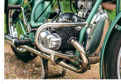
Above: Crash bars are fitted, and would help protect the cylinder heads in a tumble.
