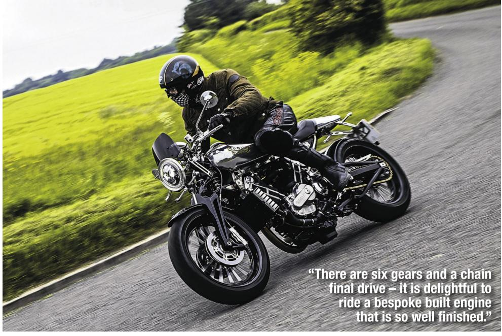
as you first see it, once you get up close few will be as cynical once you take in the details. That signature tank is 8mm cast alloy, which is then machined down to around 3mm for a perfect finish and to eradicate any possibility of a welded tank fracturing over time.
