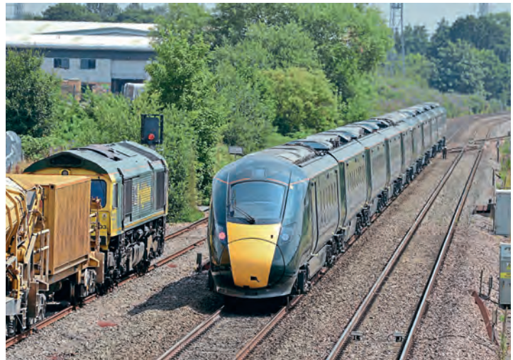
Class 802 Hitachi AT300 bi-mode trains are fitted with more powerful 938hp engines as opposed to the 750hp units fitted to Class 800/0s. On July 13, set Nos. 802001 and 802002 pass the former site of Norton Fitzwarren station with a Laira to London Paddington driver-training run, passing No. 66593 with the high-output ballast cleaner. STEPHEN GINN
