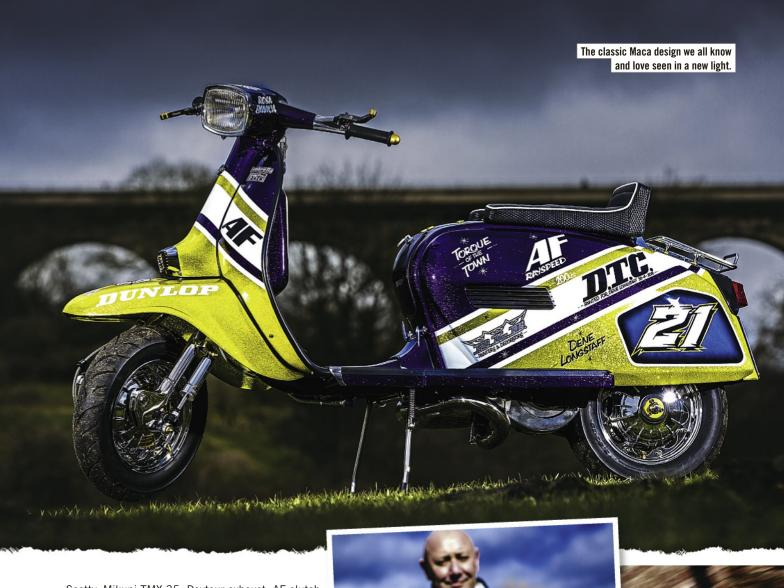
Scotty, Mikuni TMX 35, Devtour exhaust, AF clutch and Li150 gearbox with uprated sprockets. While it gives a good return of performance it's nothing too over the top and should ensure good reliability, which is required as Dene intends to use it rather a lot. The front end set up has the use of an Italian disc brake utilising a Nissin GSXR 750 caliper expertly crafted by Stewart Westgarth providing ample stopping power.
